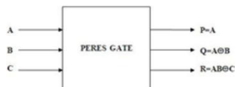
Fig 2 shows a 3 \times 3 Peres gate [4]. The input
